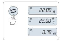
The «Series we can be used at any time to toggle between weight unit "UNIT 1", "RECALL" value (if selected), weight unit "UNIT 2" (if different from weight unit 2) and the application unit (if any).
