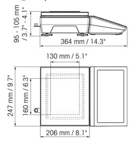
ICS4\_5 compact scale with XS weighing platform and windshield
