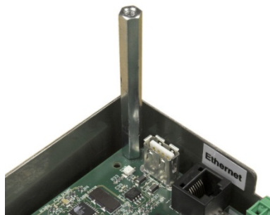
Figure 3-49: Stand-Off on Main PCB
