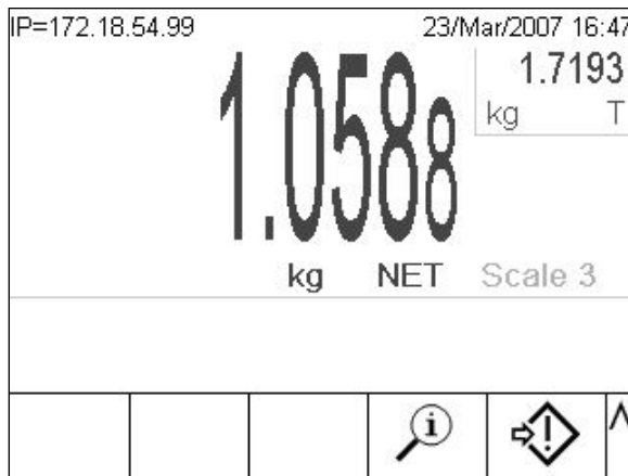
Figure 2-17: Class II-Approved IDNet Base Weight Display
